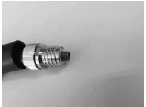
⑥ After removing the tip adapter, clean off any spatter adhered to the threads.
